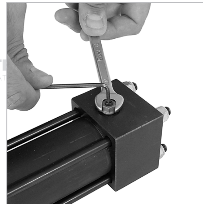
Hydraulic cylinder vent
